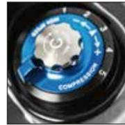
Race proven WERX cartridge with new PCS (Piston Compensator system) floating piston provides consistent damping in all conditions, eliminating cavitation
