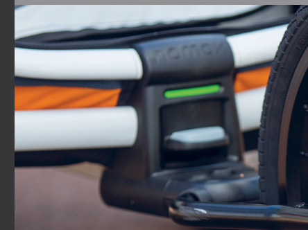
Double locked connection point in the front
