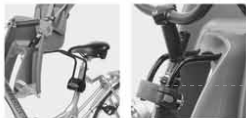
MOUNTING SYSTEM FOR REAR OPTION COMPLIES WITH EN14344
