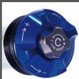
RC2: High & Low speed Compression adjust
