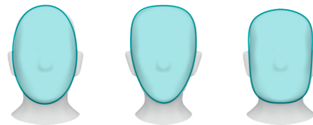
Different head shapes yet the same head circumference → Individual adjustment via uvex fit systems
