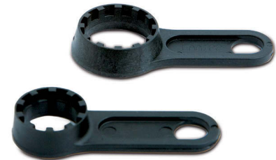
FAA122 MTB & FAA086 Trekking Preload adjuster remover. Special plastic tool to open preload adjuster caps.
