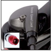
RL-R Remote speed Lock out Rebound adjust
