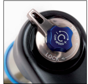
TOP DOWN: Q-LOC and rebound adjustment, clip in brake hose holder, lockout and low speed compression
