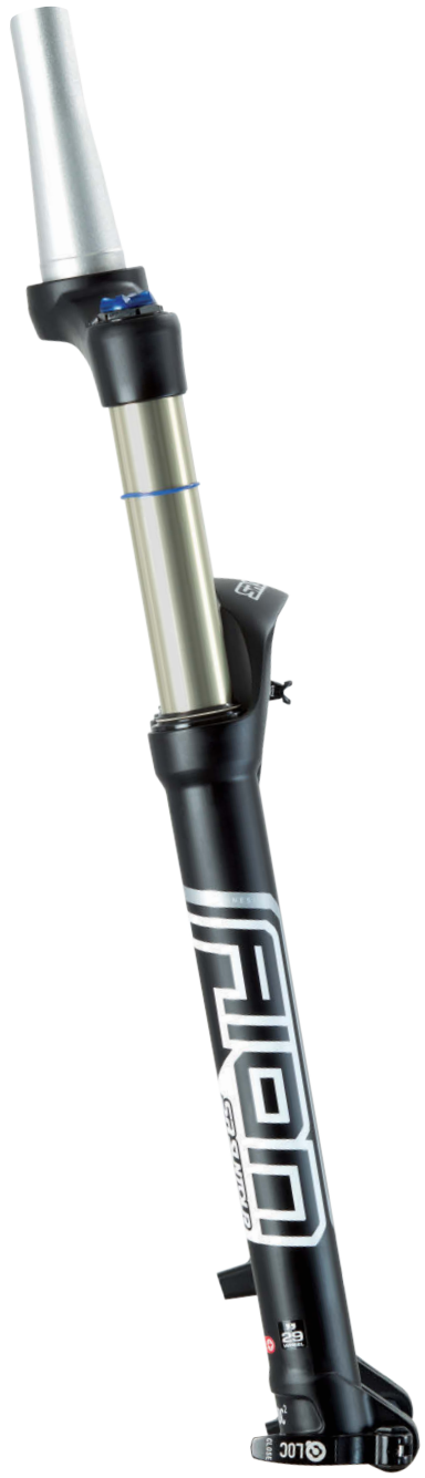
TOP DOWN: Q-LOC axle, forged aluminum crown, compression adjustment
