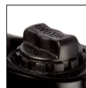
COIL W/PRELOAD ADJ. Coil spring with Preload adjuster
