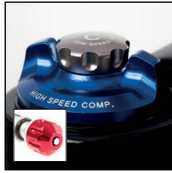
RC2 Rebound adjust High speed & Low speed Compression adjust
