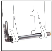
15QLC2 Diameter: 15mm O.L.D.: 100mm Weight: 112g
