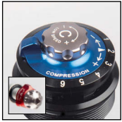
R2C2 High speed & Low speed Rebound, High speed & Low speed Compression adjust
