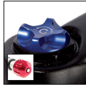
RC Reborte adjust Low speed Compression adjust
