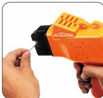
Melting and cutting cables. *Be careful the spark may hurt frames*
